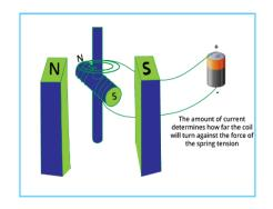
Torque on a Current Carrying Coil placed in a Magnetic field When the plane of loop is along Magnetic field
